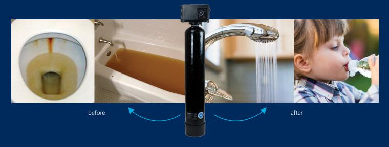
An iron problem is characterized by the red-brown staining of bathroom fixtures and laundry. The water is clear when drawn but once exposed to air the iron changes into a ferric (oxidized) state. Iron filters work by oxidizing the iron and/or sulfur and then filtering it out through the media bed.
